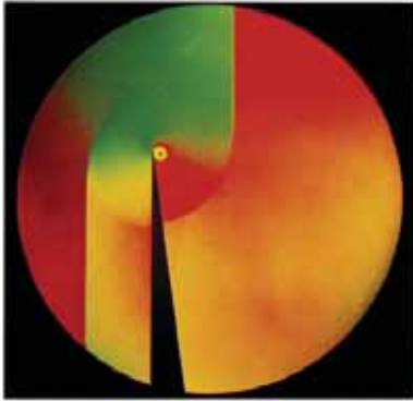
Figure 8: Color Schlieren interferogram of shock wave diffraction at a sharp edge.
